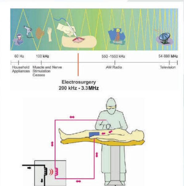
Figure 01: Applications of different current frequencies
